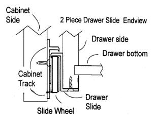
When there is a space between the edge of the stile and the cabinet side, a mechanism is needed to support the cabinet track. One option is to use a commercially available plastic rear cabinet track support as shown below.
