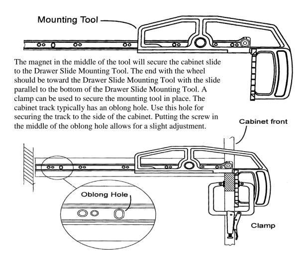
When building frameless cabinets or when the cabinet side is flush with the inside edge of the stile the cabinet track can be screwed to the inside of the cabinet as shown in the bottom left drawing.
