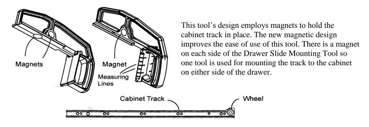
The side mounting drawer slides are made of two parts. The part that is mounted to the cabinet is called the cabinet track. It is U shaped with a flattened end to which a wheel is attached.
