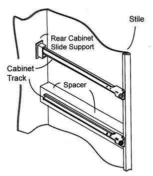
Another option is to use a wood spacer as shown above. The spacer is the width of the distance between the edge of the face frame and the side of the cabinet.
